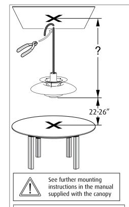
The installer must ensure to use proper means (rawplugs / screws / expansion bolts) to secure the fixture to the ceiling material. (Means not provided)
